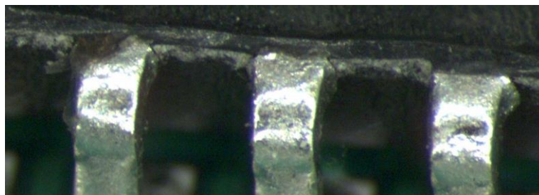
Figure 5.18-2 — Electrochemical migration between leads on a QFP
